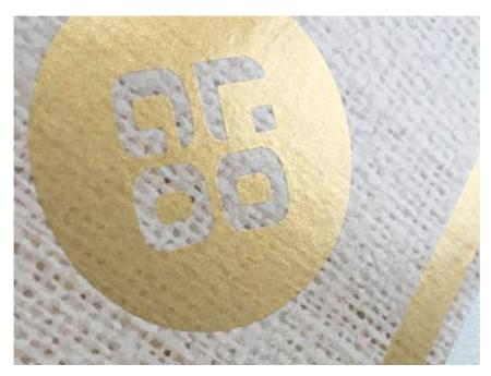
The Lumafin semi-transparent stamping foil from Kurz with translucent underprinting (Foto: Kurz)
